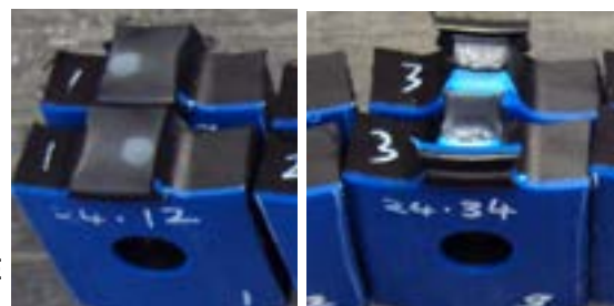
RESULT SAMPLES LEFT: BRITTLE FAILURE RIGHT: DUCTILE FAILURE
