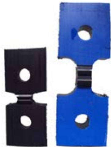
TYPE A: (BLACK) WALL THICKNESS <25MM TYPE B: (BLUE) WALL THICKNESS ≥ 25MM
