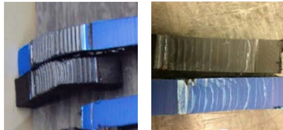
SAMPLE RESULTS: LEFT: DUCTILE FAILURE | RIGHT: BRITTLE FAILURE
